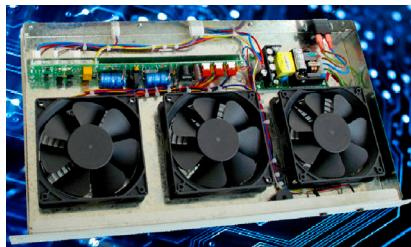
The intelligent fan trays incorporate PWM tacho fans and are designed to form part of a rack management system. They provide cooling in response to thermal requirements by increasing fan speed with temperature, against a programmable (pre-set) profile. They also offer monitoring functionality and in the event of a power, fan or control failure, will provide a remote and local alarm, by means of volt free changeover contacts, LED and buzzer.
